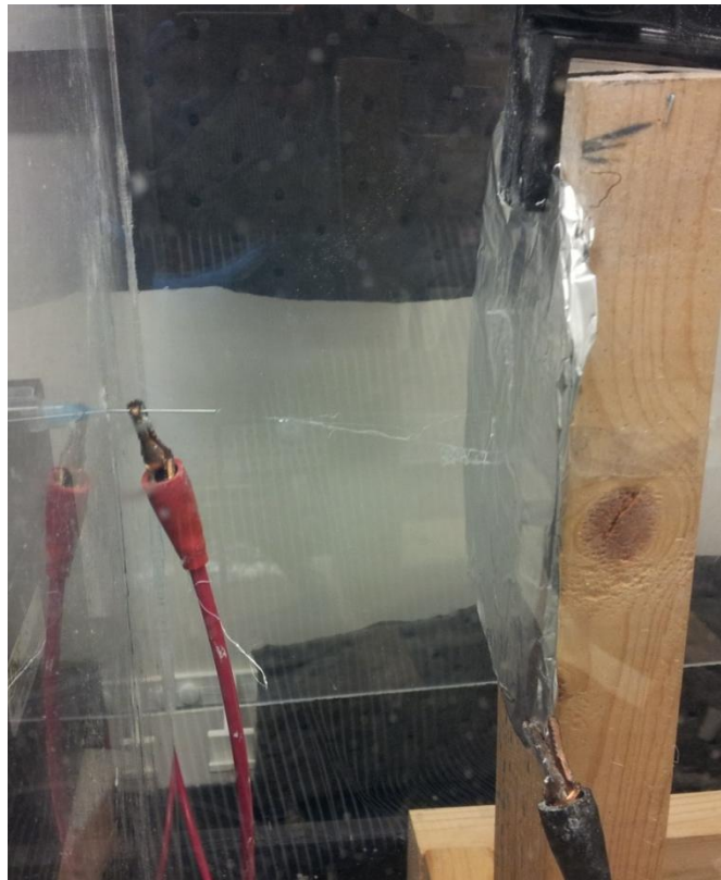
Figure 16. Image showing a fiber that formed a bridge from the dispenser to the collector.
