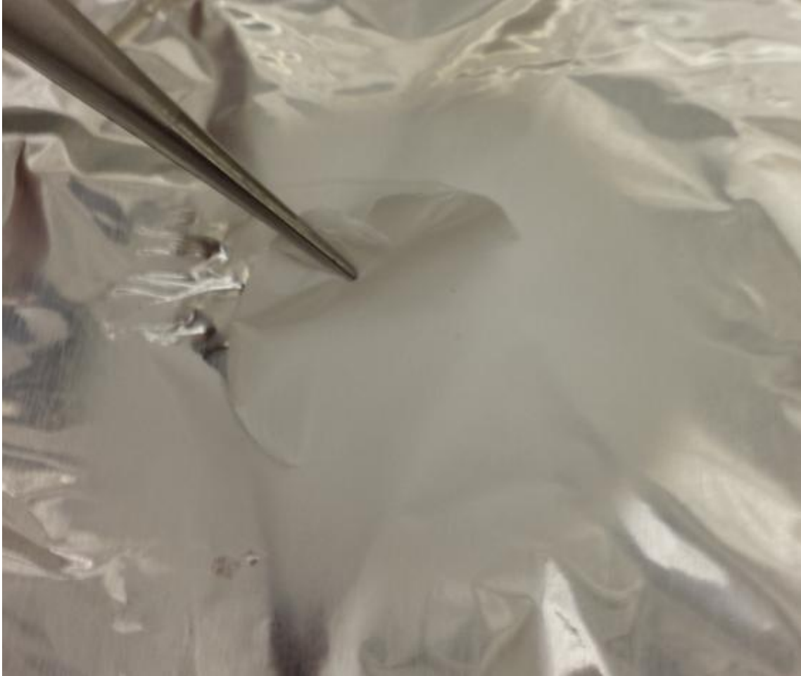
Figure 4. PVDF fiber web on an aluminum collector.
